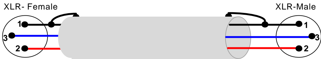
Figure 8 XLR-cable for parallel mono connection of the power amplifier.
