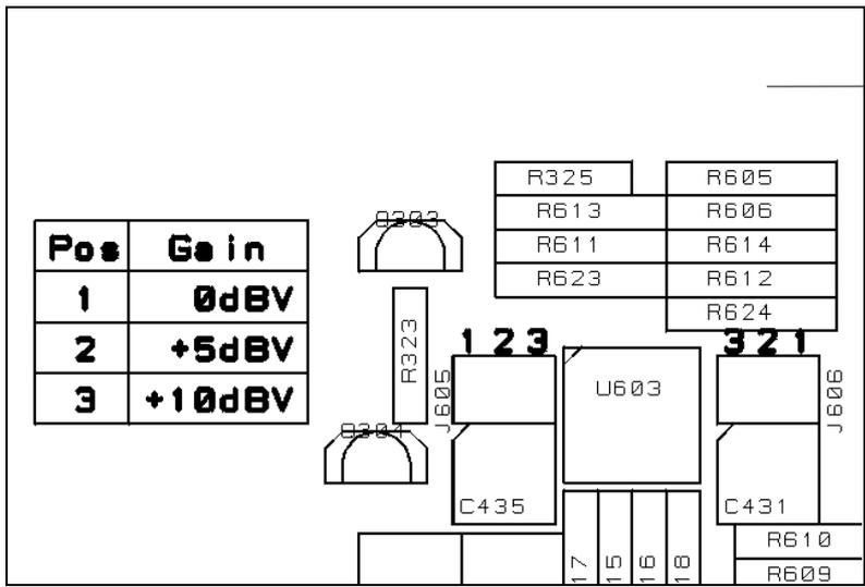
This figure shows a section of the printed circuit board including a table and straps illustrating how to pre-set the gain for the right channel.
