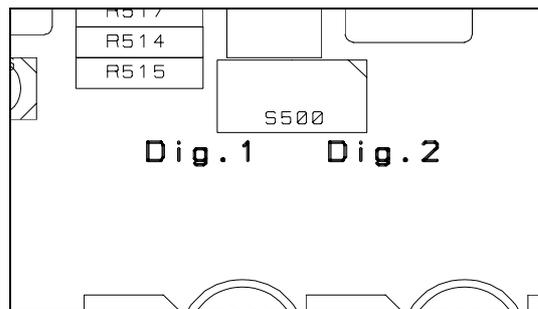
The toggle switch marked DIG.1 and DIG.2 controls which digital input is automatically selected when powering on the unit. **Please choose the position corresponding to the preferred input.**
