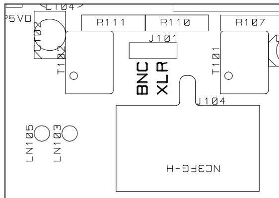
The strap section shown above is «DIGITAL INPUTS». Select between Coax 2 **BNC** or Balanced 2 **XLR**.
