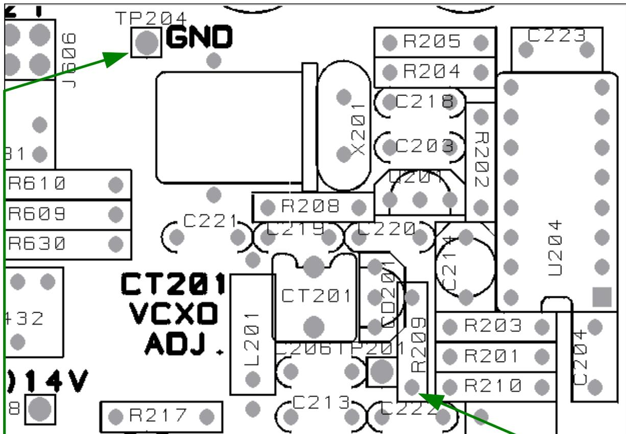
Adjust CT201 to a reading of 2.5 VDC on the voltmeter.
