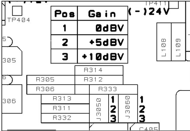
This figure shows a section of the printed circuit board including a table and straps illustrating how to pre-set the gain for the left channel.
