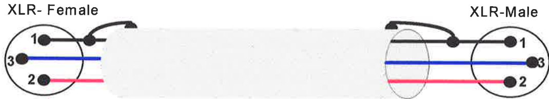
Figur 7 XLR-cable for parallel mono connection of the power amplifier
