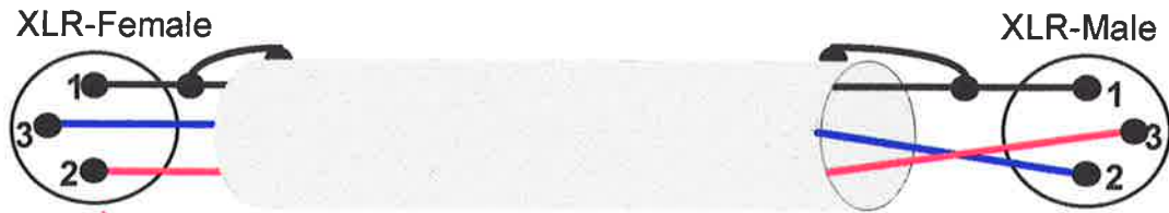
Figure 5 Special cable used to bridge the power amplifier
