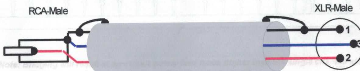
Figure 4: Unbalanced to balanced cable
