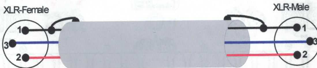
Figure 3: Balanced to balanced XLR-cable.
